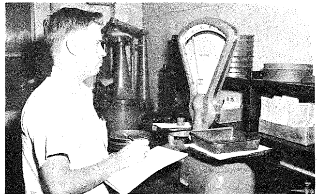
Prior to shipping, all abrasives are checked for conformance to S.A.E. size specifications. Here Harold Keene is analyzing the size distribution of a sample of shot from the boxing bins.
