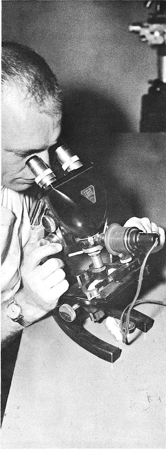
Dick Slocum checks the micro-structure of the heat treated sample for evidence of malfunctioning of a heat treating unit.
